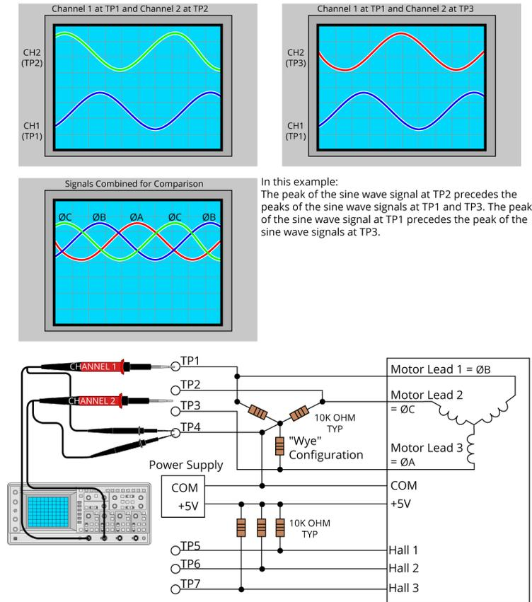
After the phase relationships of the motor have been determined, the next step is to determine the phase relationships of the Hall signals. The expected relationship between motor BEMF and the Hall signal is the peak of the BEMF. This relationship should correspond to the low voltage phase of the Hall signal. The relationship is shown in [Figure 2-6](#).
