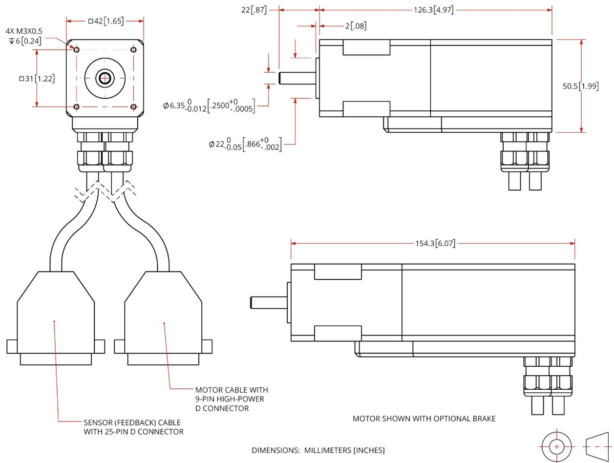
Figure 1-7: BM75, BM130, BM200 Model Dimensions (NEMA 23)
