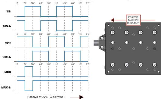
Figure 3-6: Digital Encoder Phasing Reference Diagram (Sine Wave)
