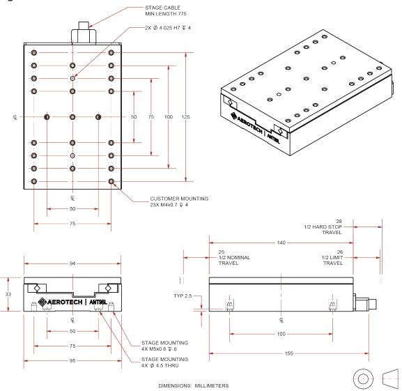
Figure 2-4: ANT95L-050 Mounting Plate Dimensions
