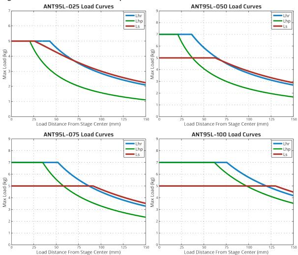
Figure 2-11: Cantilevered Load Capabilities
