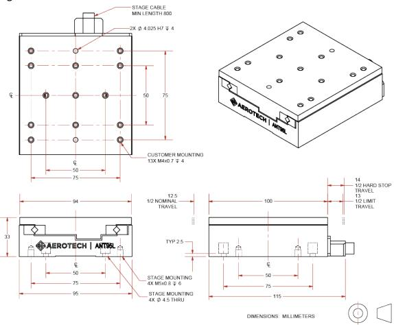
Figure 2-2: ANT95L-025 Mounting Plate Dimensions
