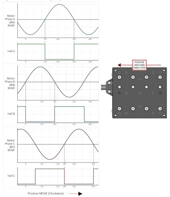
Figure 3-5: Encoder Phasing Reference Diagram (Standard/Square Wave)
