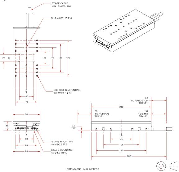
Figure 2-8: ANT95L-100 Mounting Plate Dimensions
