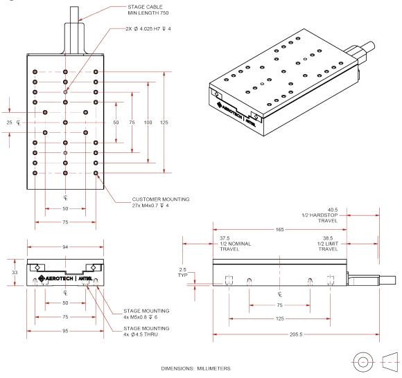
Figure 2-6: ANT95L-075 Mounting Plate Dimensions
