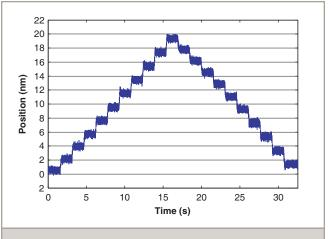
ANT130V-5-PLUS 2 nm step plot. Best-in-class resolution and exceptional in-position stability for large travel stages.
