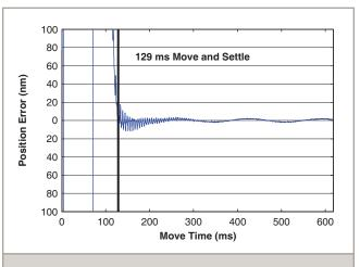
ANT130V-5-PLUS step and settle performance at 75 mm/s, with a settle spec of  $\pm 20$  nm, and a step size of 5 mm. Outstanding settling time enhances throughput of most applications.
