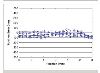
ANT130V-5-PLUS accuracy and repeatability. This multiple test run over an extended period of time shows the high level of system accuracy and repeatability.
