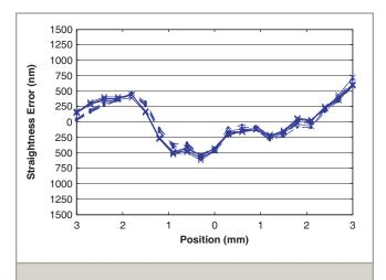
ANT130V-5-PLUS straightness error, five runs, bi-directional, parallel to the wedge.
