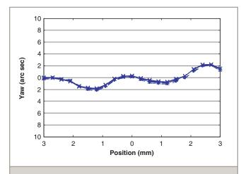
ANT130V-5-PLUS yaw, five runs, bi-directional. Highly repeatable, minimal yaw error enhances system positioning accuracy.
