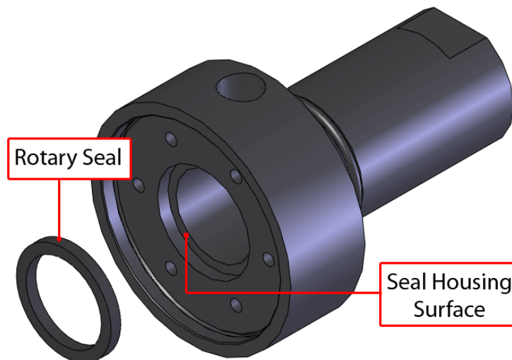
Figure 4-11: Seal Housing Location
