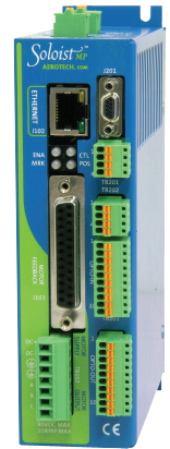
Soloist MP Width: 41.1 mm Height: 141.2 mm
