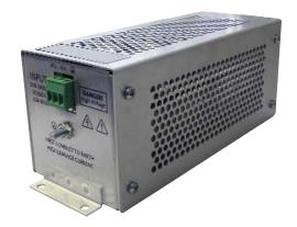
Aerotech's UFM noise filter module is used to reduce conducted line noise generated by switching servo amplifiers. The UFM is used with any BA series amplifier to conform to CE noise directives.
